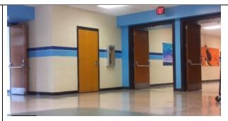
The fire doors in this video automatically close, because the electromagnet holding them open is released by the fire alarm. Click on the picture above to see the fire doors close automatically. Students can complete a <u>See Think Wonder</u> <u>Template</u> after watching the video.
