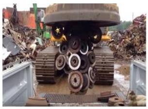
Click on the picture to view how an electromagnet is used to pick up large pieces of metal. Electromagnets are devices that create a magnetic field through the application of electricity. Wrecking yards employ extremely powerful electromagnets to move heavy pieces of scrap metal or even entire cars from one place to another. Students can complete a <u>See Think</u> <u>Wonder Template</u> after watching the video.
